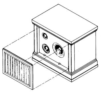
The AS35 is a furniture style "air suspension" sealed speaker system incorporating a high compliance 12" bass driver, a 4" high compliance closed back midrange and a wide dispersion 1" super dome tweeter.
